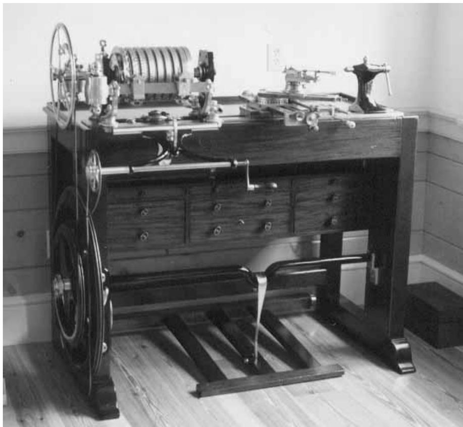
Figure 12: Rose engine lathe (image courtesy of John Edwards)
