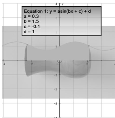
Figure 7: Woodturned vase curve modelled in Autograph
