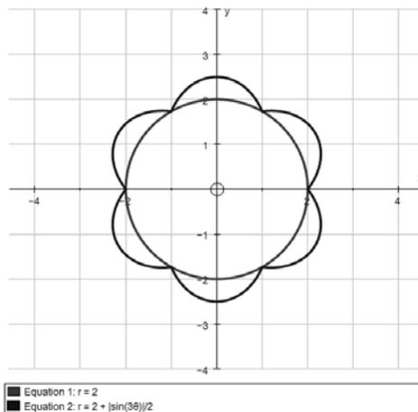
Figure 14: Rose engine bowl cross-section
