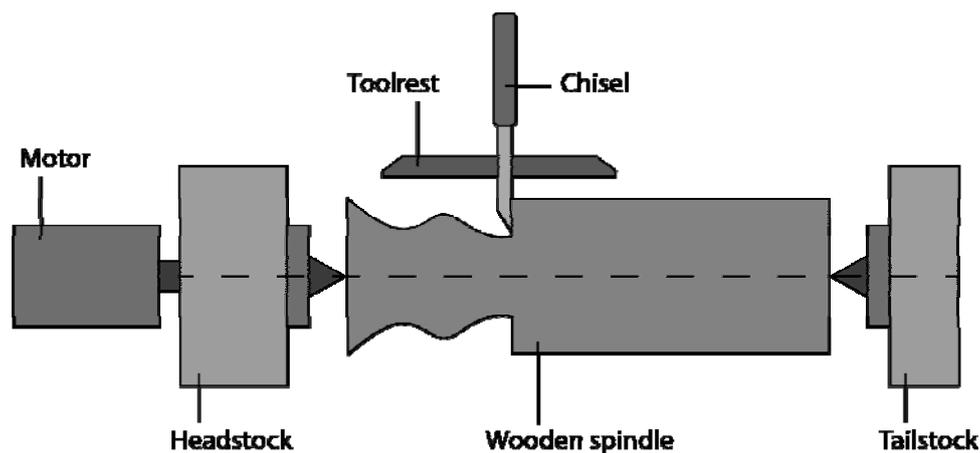
Figure 3: Lathe diagram
