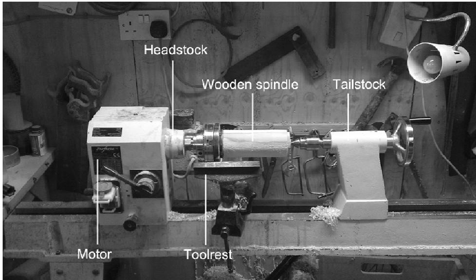
Figure 1: Parts of a Lathe
