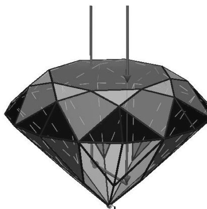
Figure 4.4: Circular brilliant cut with regular optical path
