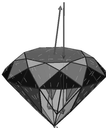
Figure 4.3: Circular brilliant cut with non-regular optical path
